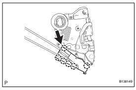
(d) Insert the door lock open rod into the front door lock, then set it to the door panel.
